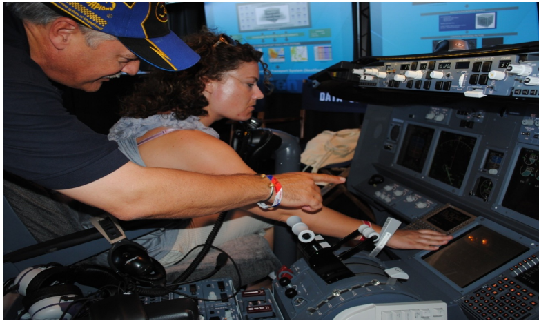
FAA NextGen Data Communications Team Member Jerry Smith points out the cockpit display unit (CDU) on the Data Comm Boeing 737 flight simulator to an Oshkosh AirVenture participant. The CDU receives information and instructions digitally from air traffic controllers. This significantly reduces voice communication errors, improves efficiency, and reduces controller and air crew stress.
